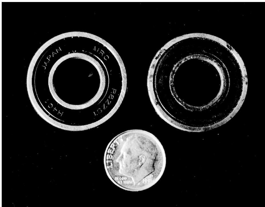
Figure 7 Corrosion of bottom plate bearing from a biofilm annular reactor. The bearing on the right came from a reactor that grew sulfate-reducing bacterial biofilms. A clean bearing is shown for comparison (left). The bearings are 2.7 cm in diameter.
